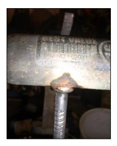
Clamp the nail upright in a vice with a little silver solder (NOT LEAD TIN SOLDER) and flux in the groove.
