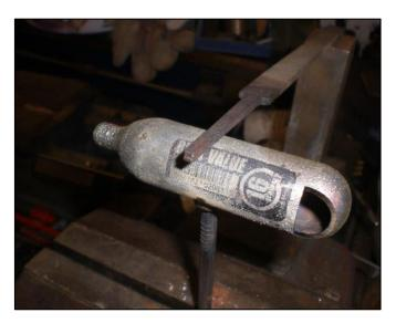
With a half round file cut a groove in the head of the nail to suit the diameter of your cartridge.
